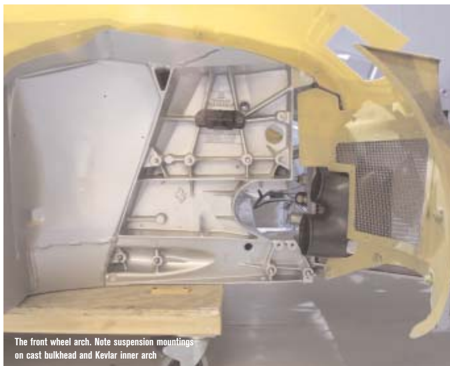
The aluminium chassis with the engine removed
