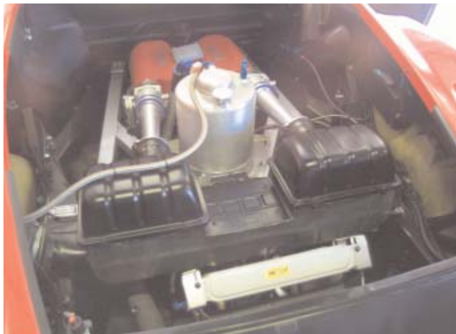
The all alloy Ferrari V8 nestles deep in the 360's engine bay - it produces 430bhp at 8500rpm and 275lb.ft at 4750rpm
