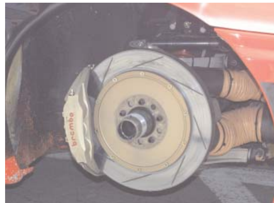
Front and rear brakes are racing spec courtesy of Brembo while the suspension is standard Ferrari 360 Modena
